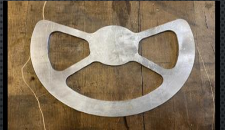
Figure 10: Steering Wheel Cut Using Tormach
