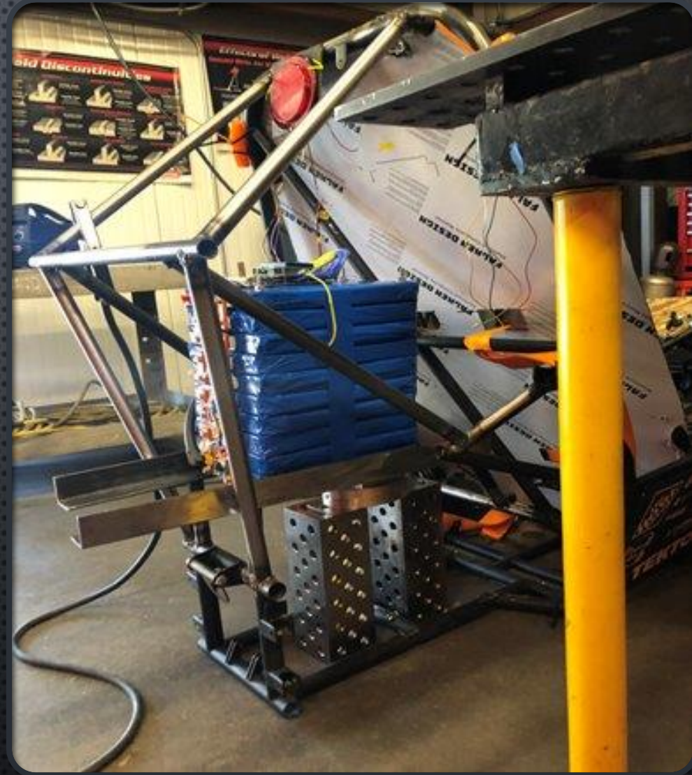
Figure 5: Battery Mount Test with failure safety devices
