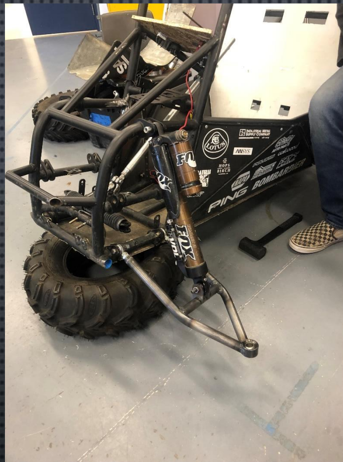
Figure 7: Lower Control Arm Fitment
